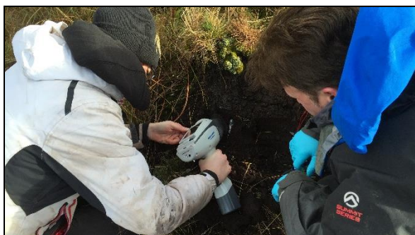
Experimental deployment of field portable XRF in the vicinity of a former homicide grave (Photo: Dr Laurance Donnelly. Equipment, Ms Carole Davenport, John Moores University, Liverpool, UK).
