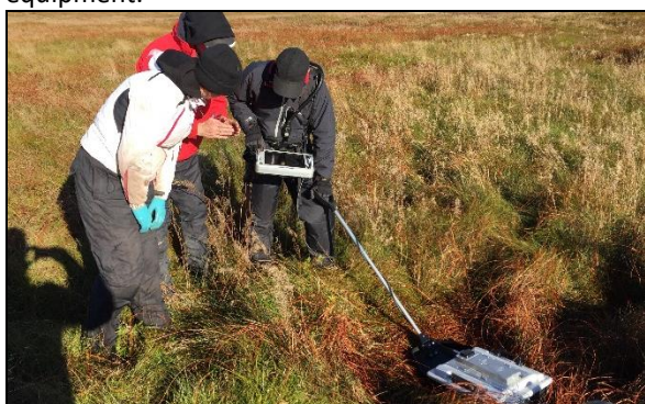
Experimental GPR for a grave search (Photo: Dr Laurance Donnelly. Mala geophysical supplied courtesy of Mr Mike Langton. Geophysics support from Dr Alastair Ruffell).
