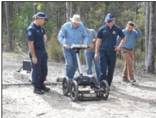
Field applications of EM38 and GPR, Australian Federal Police Training Centre, in Brisbane, Australia
