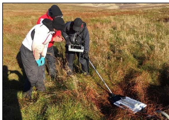
Experimental use of ground penetrating radar to over a control site associated with an unknown grave, in the north of England (Photo: Laurance Donnelly. Mala geophysical supplied courtesy of Mr Mike Langton. Geophysics support from Dr Alastair Ruffell)
