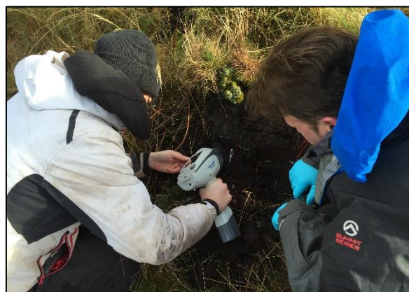
Experimental deployment of field portable XRF in the vicinity of a former homicide grave (Photo: Dr Laurance Donnelly. Equipment, Ms Carole Davenport, John Moores University, Liverpool, UK)
