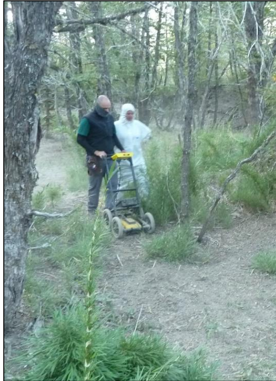
IUGS-IFG Crime Scene Adviser, Prof Pier Matteo Barone, using Ground Penetrating Radar as part of a ground search (Photos: Pier Matteo Barone)
