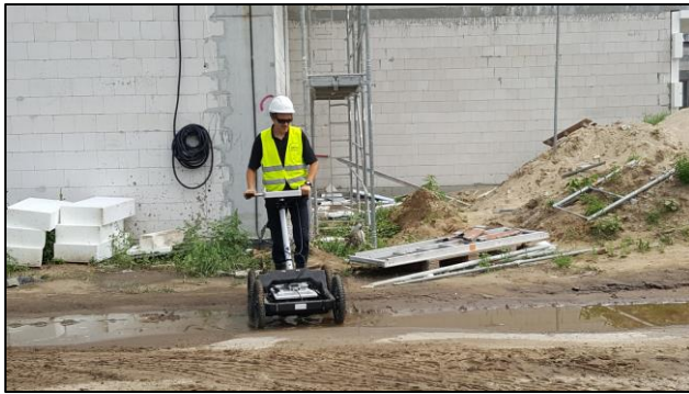
Ground searches of two sites in Poland, using ground penetrating radar, for suspected Second World War mass graves related to genocide (Photos: Michal Pisz).
