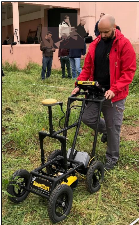
IUGS-IFG Crime Scene Adviser, Prof Pier Matteo Barone, using Ground Penetrating Radar as part of a ground search (Photos: Pier Matteo Barone)
