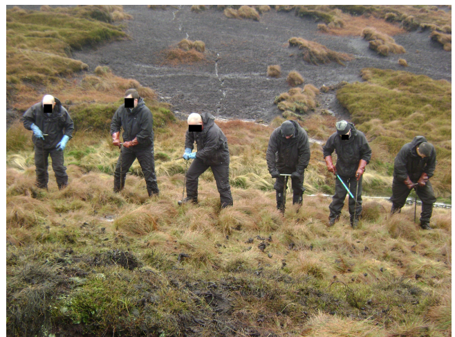
Figure 12. Line of search trained police officers auguring to locate a burial in Europe (Photo: Laurance Donnelly).
